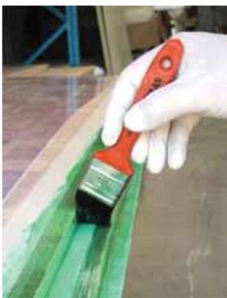
Prior to applying adhesive to the Z-Joint, carefully remove approximately 25mm of peelply from the outside edge of the male scarf, taking care not to damage the laminate. Scarfs should be brushed with a clean brush to remove dust and any contamination that would inhibit adhesion.
