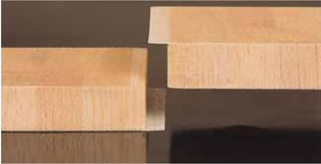
Particularly in strength critical applications the Z-Joint must be given adequate consideration. It can be considered analogous to a weld in aluminium, as a strength reduction exists.
