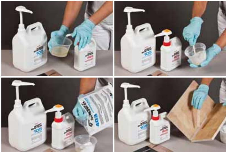
If you are going to be using the mixture out of a roller pan, mix it thoroughly in a mixing pot before transferring it to the roller pan. **DO NOT USE** a power mixer unless you thoroughly scrape the sides and corners of the mixing pot while mixing.
