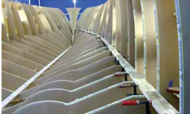
CNC-routed plywood, or MDF jigs can be supplied by vDL Composites
