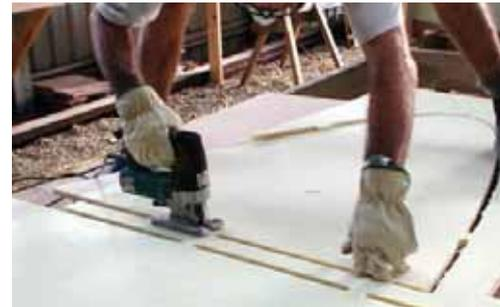
Each pre-cut part is left attached to the panel by small tabs to ensure the kit arrives with all components securely in place. The tabs are easily cut away, when the panels have been joined.
