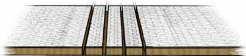
Initially determine the desired internal angle, and outer corner radius. Following the calculations below, will provide the required details on number of slots, and their spacing, to achieve the required curve.
