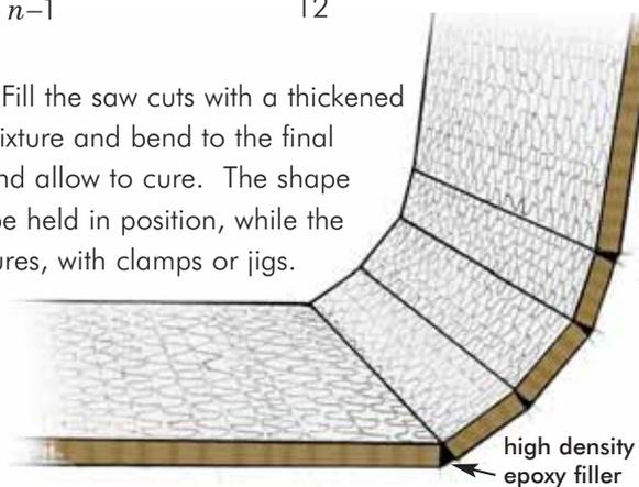
**Step 3:** An additional layer of fibreglass cloth is applied to the inside of the curve with an epoxy laminating system, covering all the slots and overlapping the end slots by 30 – 40mm.
