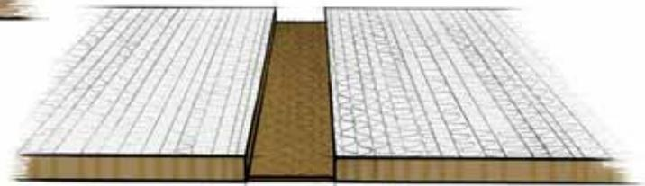
**Step 2:** The cut should be filled with a mixture of WEST SYSTEM 105 resin with 206 Slow hardener, modified with 409 Microsphere Blend. This combination will produce a strong, waterproof bond that will hold the curve when cured.
