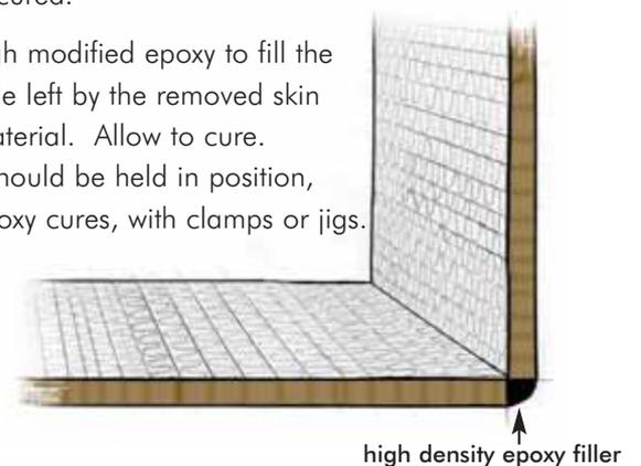
**Step 3:** Fill the internal angle, with a 20mm radius of modified epoxy and allow to cure. Apply an additional layer of fibreglass cloth to the inside of the angle, overlapping the fillet by 25mm on each side.
